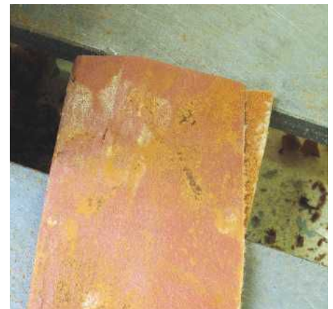
▲ Pic.9 An oily timber like padauk can be a nightmare to sand, evidenced by this clogged piece of 120 grit. Keep using a different area on the abrasive or you will generate too much heat
